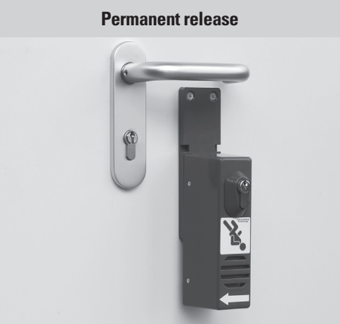
With the device key, the GfS ExitControl can be brought into a permanent release position without alarm by turning it 180°. In this position, the door can be entered normally.
